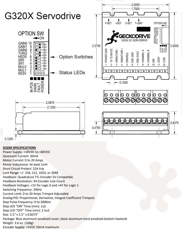
Pulse Multiplier: 1, 2, 5, or 10 times input step rate
